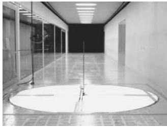
Photo 9 Measurement of wind force and moment to the Support pole without test net
